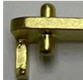
In-die counter boring with tilted angle
